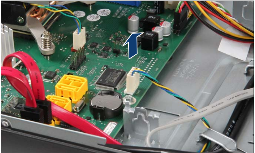
Figure 81: Disconnecting the cable of the system fan module
